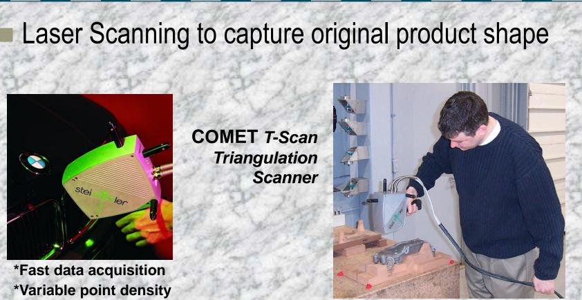
\*Linetracking (feature lines, contrast lines, border lines, edges, holes, ...) \*High dynamic range allows to capture surfaces with different and variable optical properties.
