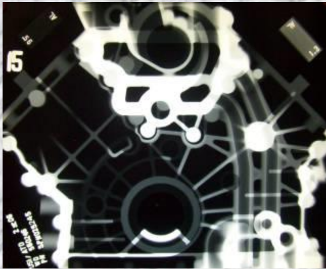
X-Ray inspections for internal shape defects
