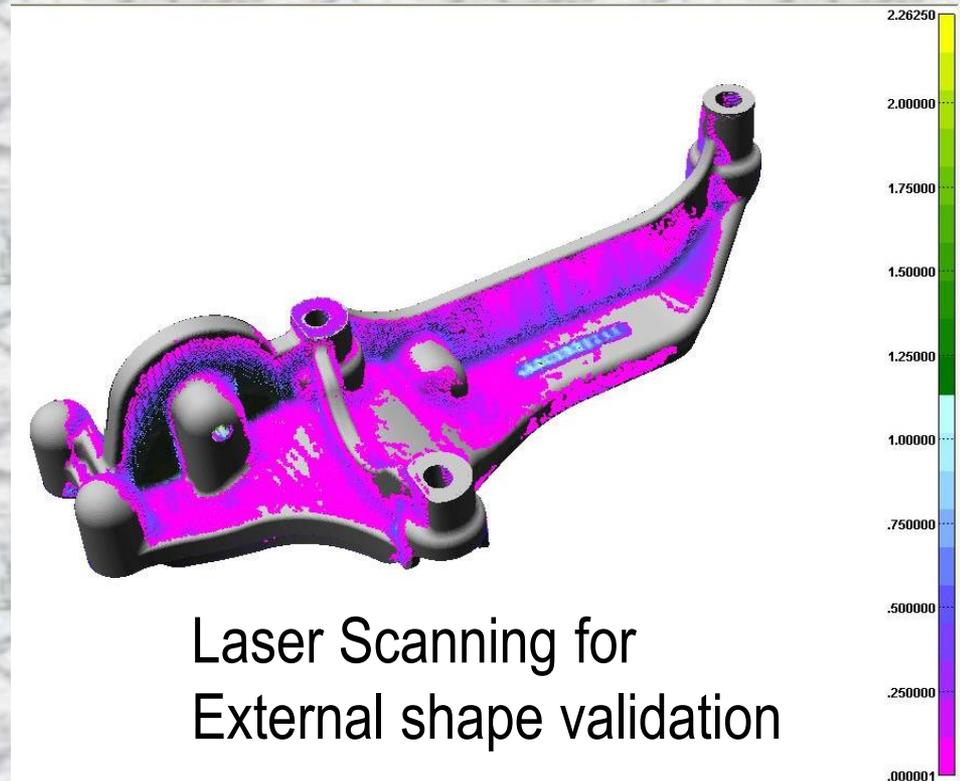
Laser Scanning for External shape validation
