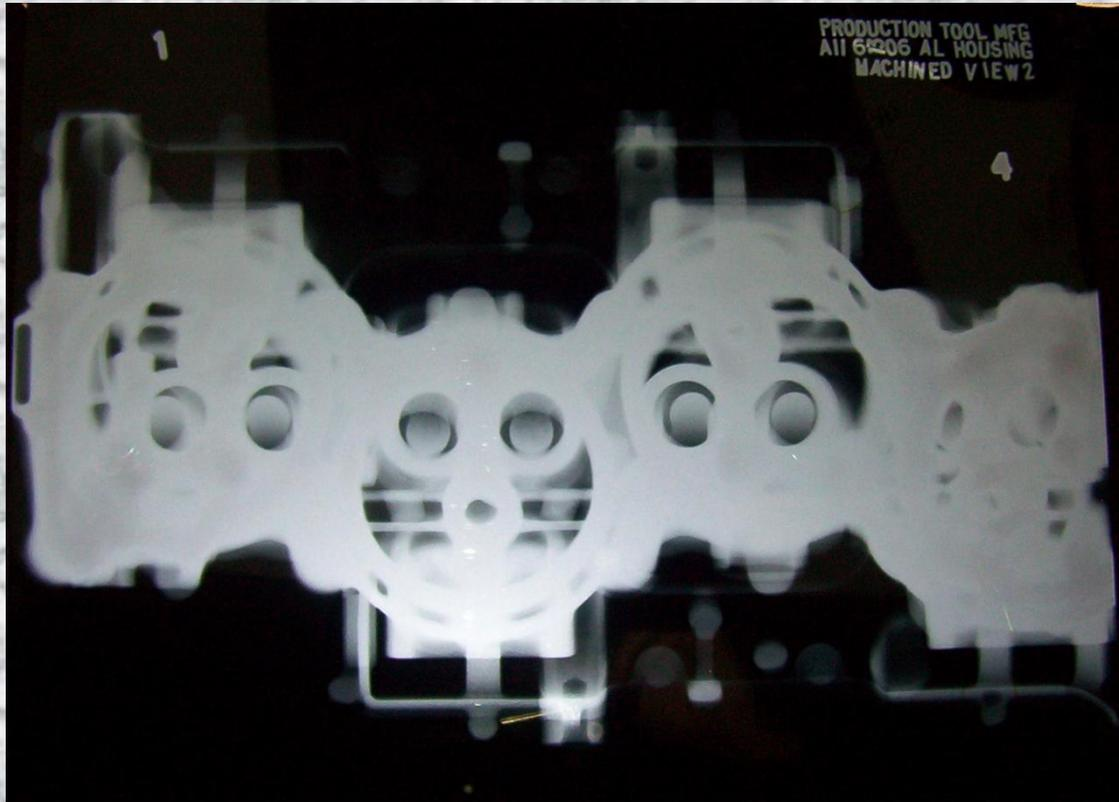
X-Ray inspections for internal shape defects
