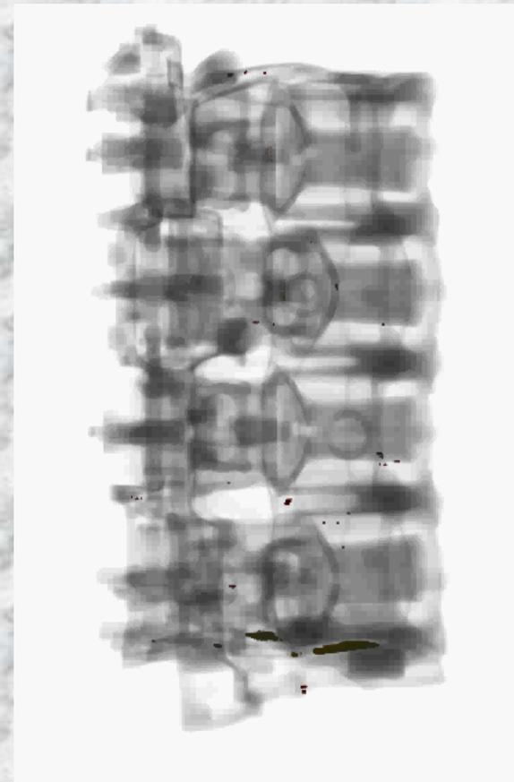
CT Scanning inspections for internal & external defects
