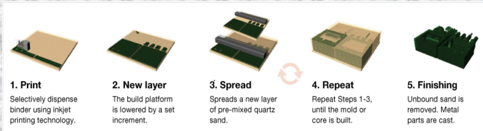
Rapid Casting Technology (RCT) offers unprecedented flexibility to produce complex, finely detailed, patternless castings. While reducing production costs and time to market, RCT eliminates the need for physical tooling to produce a casting. By removing the constraints of hard tooling, this allows extreme casting design to become a reality.
